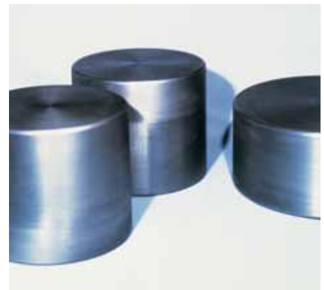
Molybdenum billets weighing approx. 1000 kg
