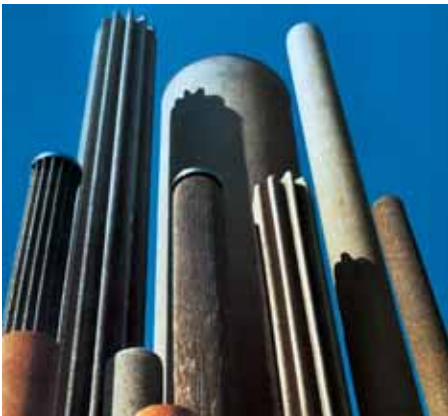
Metal filters produced to net shape
