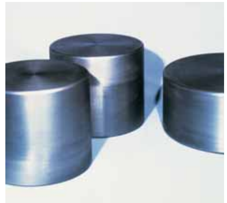
Molybdenum billets weighing approx. 1000 kg
