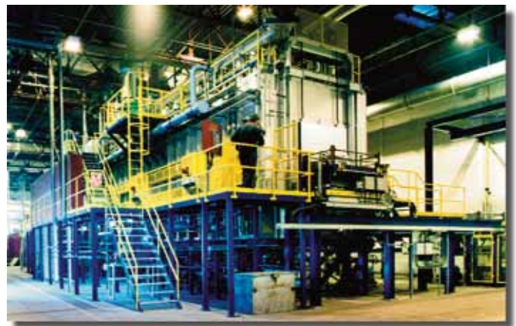
4d. Dual level roller hearth Sand Lion® systems for engine blocks T-6 heat treatment.
