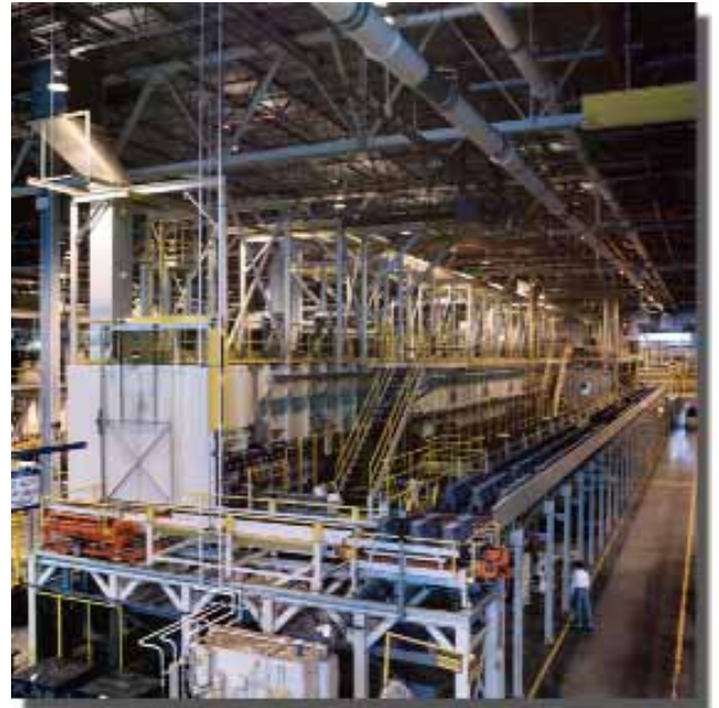
4b. Closed loop, fully automated Sand Lion® system designed for processing of up to 90 I-4 engine block castings per hour. The system includes robotic loading of castings, water mist air quench and 26 tons per hour sand reclamation capacity.
