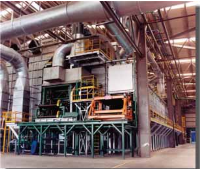
4c. 3-in-1 continuous U-shaped T-6 solution heat treatment system with both air and water quench capabilities.
