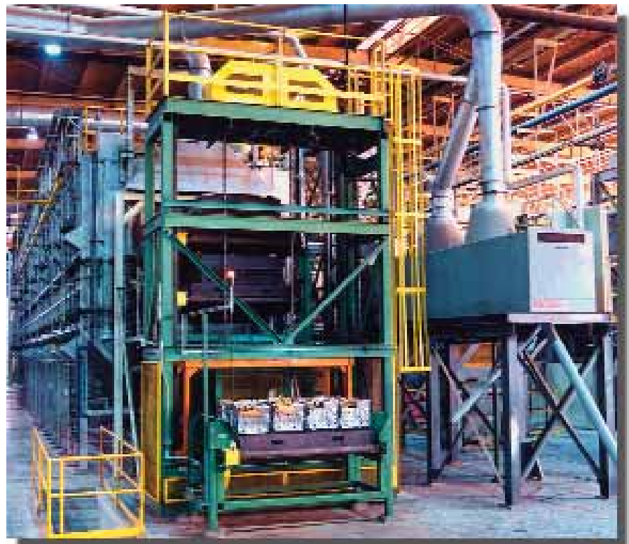
3b. 3-in-1 continuous U-shape T-6 solution heat treatment system with air quench and water quench systems. It also reclaims 15 tons/hour of silica sand to a controlled L.O.I. of less than 0.08%.
