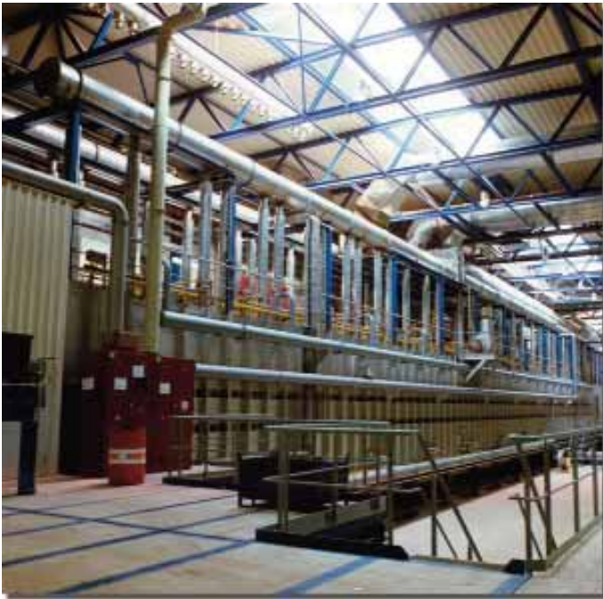
4a. Continuous Sand Lion® roller hearth system installed in Germany. This system has the capacity to heat treat 6 to 8 engine block castings on a tray, up to 160 castings per hour.
