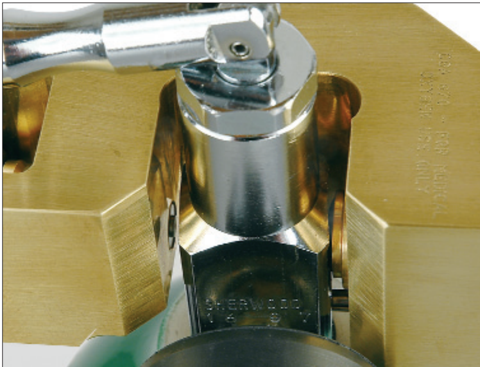
Figure 8. Valve properly aligned.
