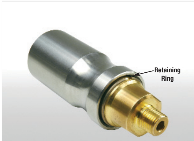
Figure 41. Check retaining ring to make sure it is tightly seated in its groove.
