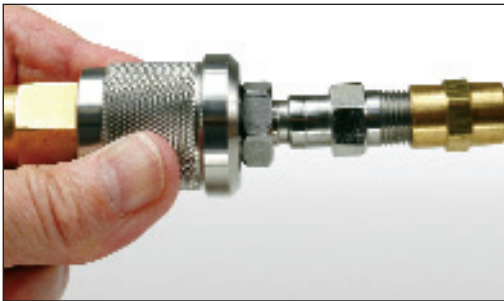
Figure 23. Coupler properly aligned.
