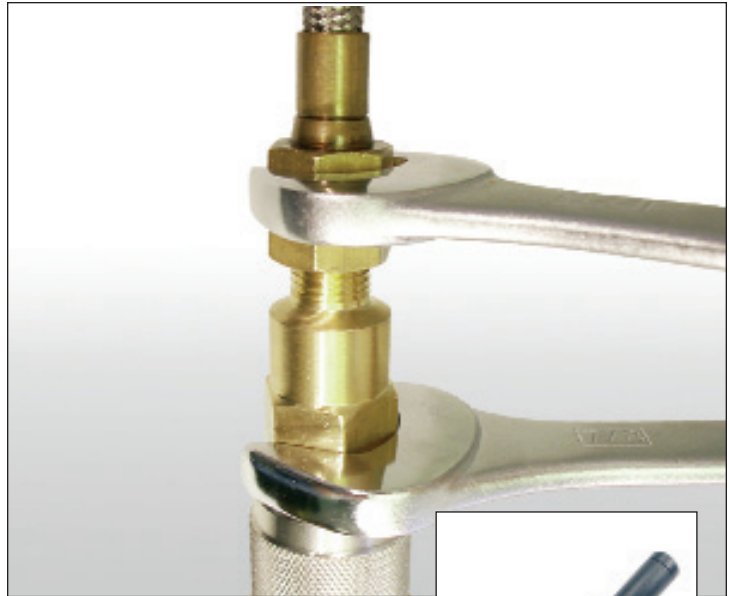
Figure 1. Torque to maximum 15 ft-lb.
