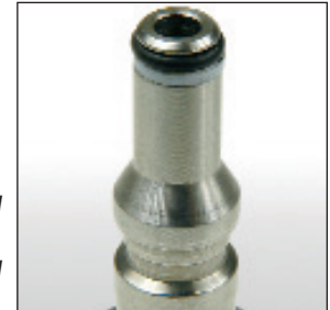
Figure 42. Make sure coupler does not thread apart. Examine the connector length and thread tightness periodically. The threads should be tight to 10ft-lbs between the front and rear hex.
