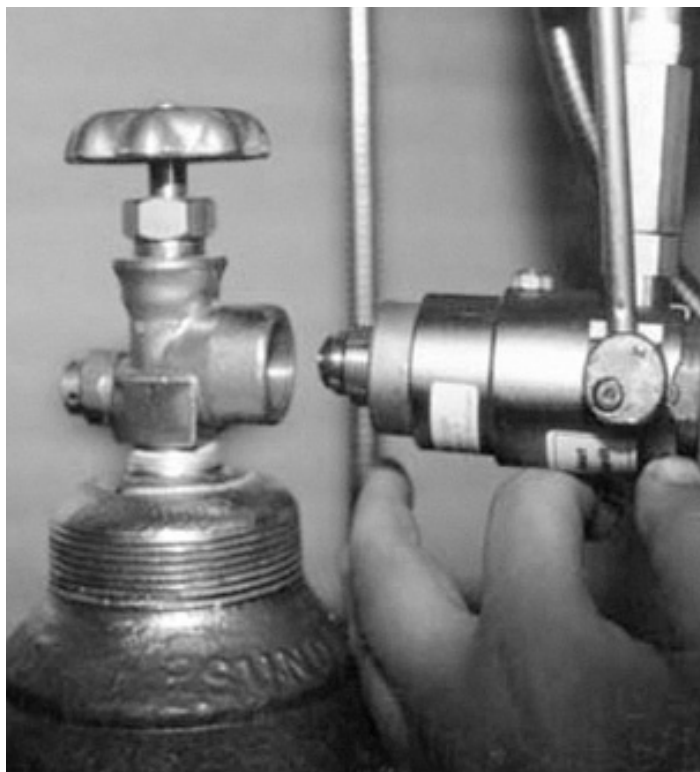
Insert connector into valve...flip handle...DONE!
