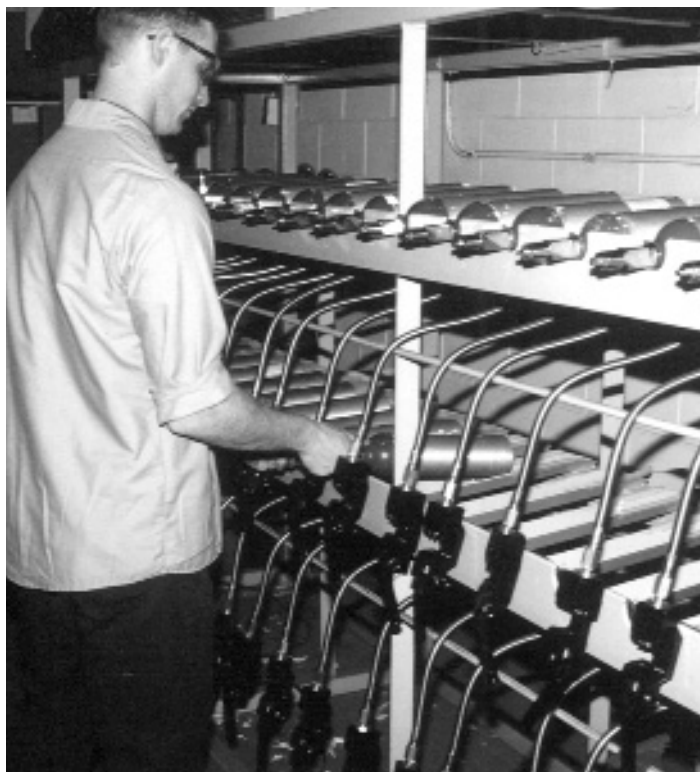
MediMates on inverted medical oxygen rack filling application.
