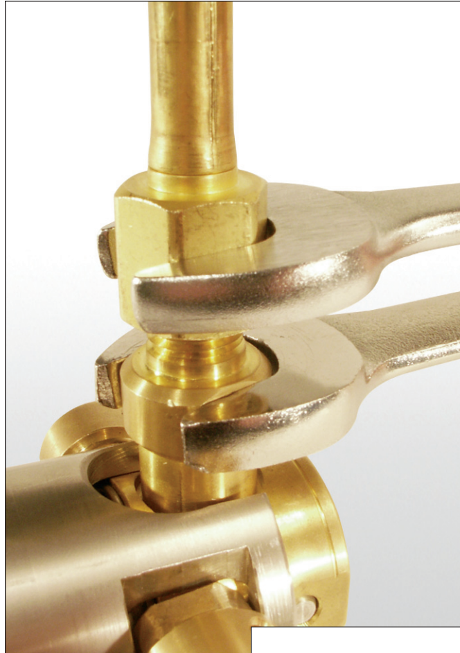
Figure 1. Torque to maximum 15 ft-lb.
