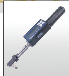
Figure 19. If screws are loose, tighten to 7 ft-lb.
