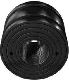
Standard glass-filled Teflon, O-ring energized piston seal with two bronze-filled bearing strips—installed on a ductile iron piston. (Code G)
