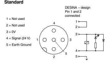
Pins are as seen on valve (male pin connectors).
