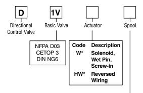
\* Valve schematic symbols are per NFPA/ANSI standards, providing flow P to A when energizing solenoid A. Note operators reverse sides for #008 and #009 spools. See installation information for details. To configure per DIN standards (A coil over A port, B coil over B port) code valves as D1VHW\*\*\*.
