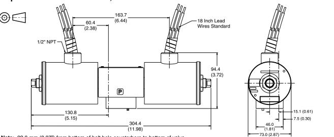
Note: 22.0 mm (0.87") from bottom of bolt hole counterbore to bottom of valve.
