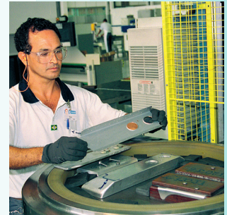
Aerospace parts formed in an Avure Flexform press at Embraer in Brazil.
