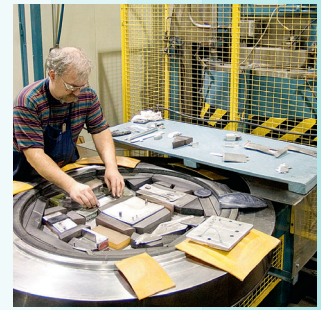
Aerospace parts made in an Avure Flexform press at the Cessna Aerospace Company, in Wichita, KA, USA.
