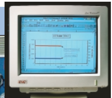
Superheated steam cycling test in progress (950°F - 1800 psig / 510°C - 124 bar). 1000 cold and 1000 thermal cycles with 1000°F (538°C) superheated steam and five blowdowns with "0" leakage.
