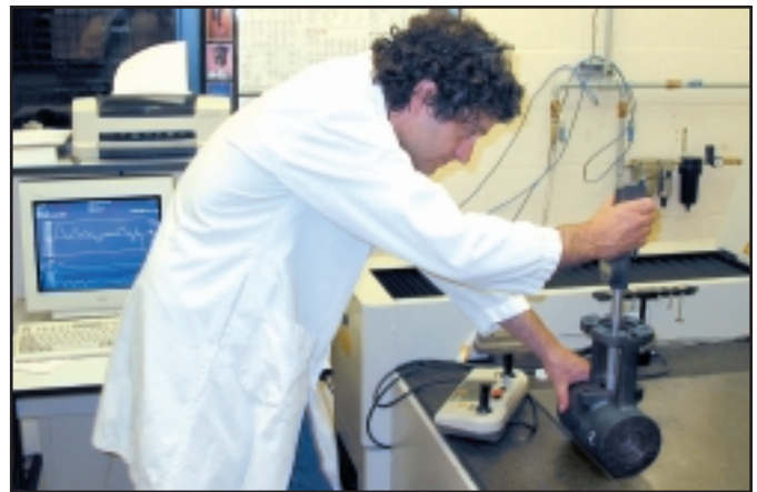
Velan performs statistical process control to monitor tool wear and concentricity of bores, during the manufacturing process.
