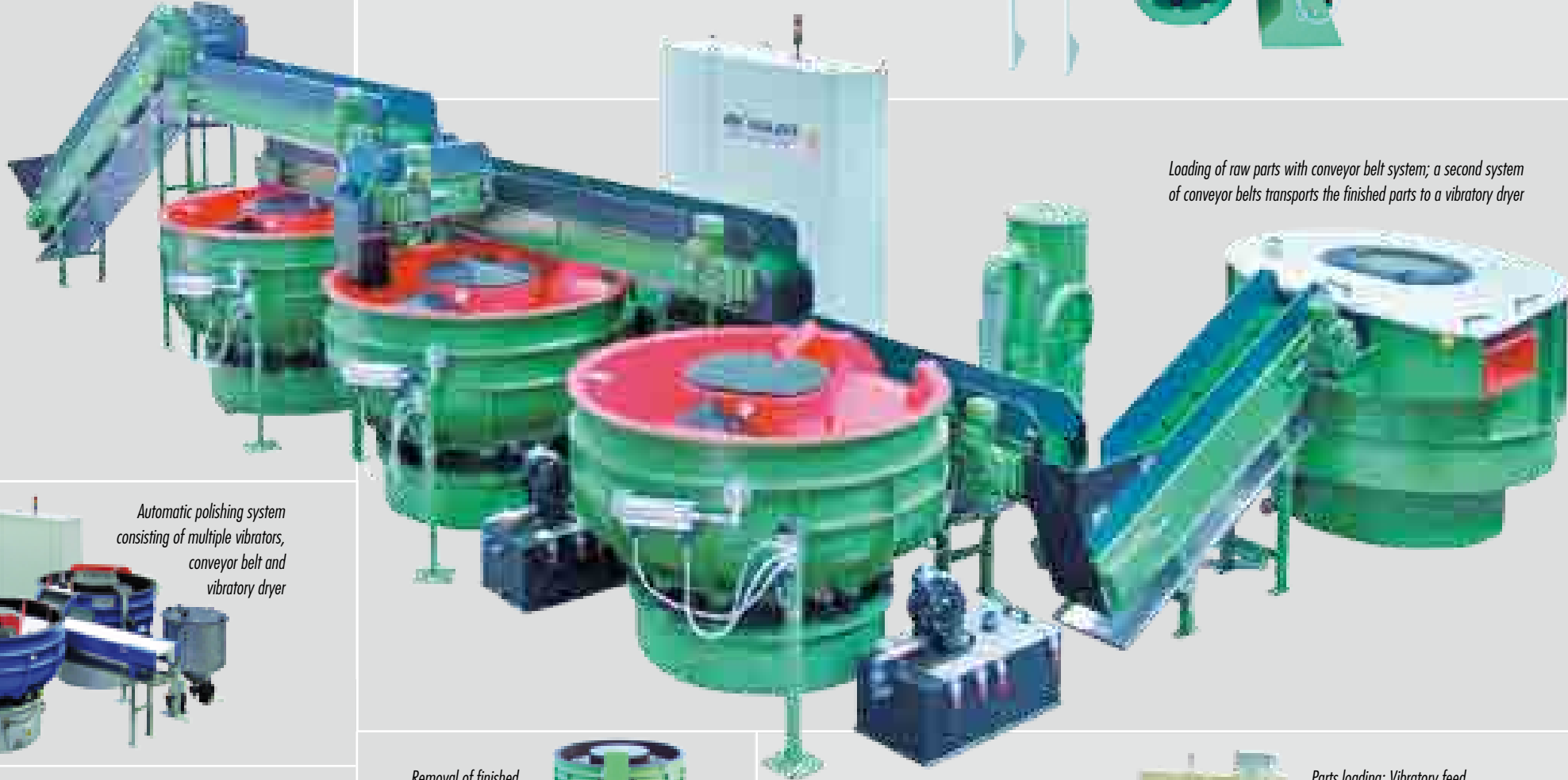
Removal of finished parts and media from work bowl with pneumatic unload gate; external separation with magnetic drum; drying in vibratory dryer
