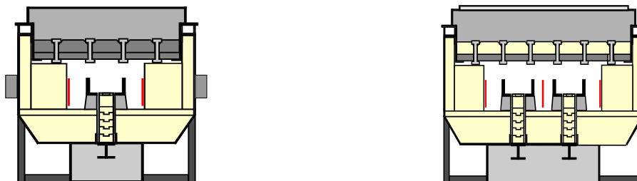
Cross section view of a conventional high-temperature sintering zone (left) and the sintering zone of a “twin runner” (right)
