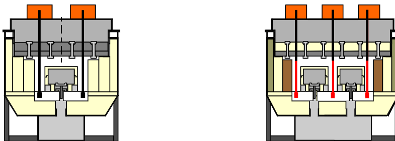
Cross section view of a stearate zone with a single and double walking beam
