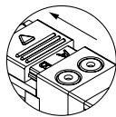
Manual override switch unlocked status
