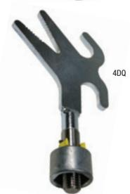
The **MECHANICAL HAND STICK** serves both as a hand and as pliers so that any serve-up or type of tie can be made or removed from the line. Very little effort is required to serve a wire taut and as perfectly as when hand and pliers are used. It is possible to roll the wire into place around the conductor, making a tight connection easily, instead of jerking and pulling.
