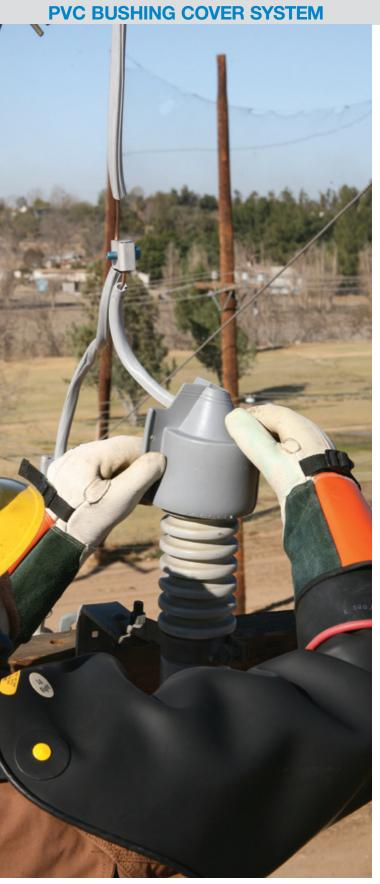
**COMPLETE BUSHING-STINGER COVER** This product is made from UV resistant PVC plastic to maximize the outdoor durability. The Complete Bushing/Stinger Cover interlocks with the top weather shed of the bushing and securely fastens by inserting lock buttons (provided). The Complete Bushing/Stinger Cover can be installed without disconnecting equipment using rubber insulating gloves. This product offers an integrated stinger cover which will cover the lead wire for an easy solution.
