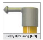
**SWITCH STICKS** use closed cell foam filled tubular fiberglass made in accordance with ASTM Standard F711. Both the standard head and the heavy duty prong disconnect are made of durable high strength aluminum bronze alloy.
