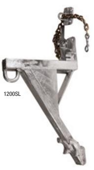
**CROSS ARM GINS** are used on cross arms when only one conductor needs to be raised. Use the arm gin to change insulators; apply an armor rod to a conductor; raise a conductor from a lower position to the cross arm, or lower the conductor. The 2-1/2" (6.4 cm) diameter fiberglass pole has two eyes at the top in which to hook the block line and tie back line. The base fits a 4-3/4" x 5-7/8" (12.1 x 14.9 cm) cross arm. Included shims are needed for smaller arms.
