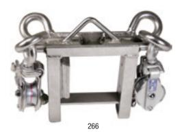
**FABRICATED ARM SLINGS** are used as an all-purpose sling for nonenergized and live line work, the fabricated arm sling is made to fit snugly over the arm by using the filler plates (included) to adjust the opening. Weight - 6 lbs. (2.7 kgs).
