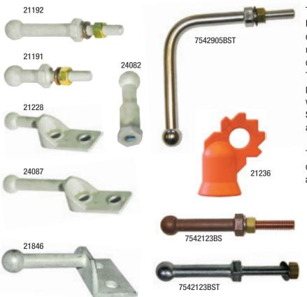
The **BALL STUDS** and the **OFFSET NEMA PAD BALL STUDS** are made from tin-plated copper alloy or copper. They each have a 1" (25.4 mm) diameter ball. Recommended installation torque of 300 in. lbs. The short stud is used conventionally. The long stud can also be used as the grounding point for "C" or Duck bill clamps that have a jaw width of 2.75" or less. The Offset Nema Pad Ball Stud has the standard Nema bolt hole spacing and also comes in both long and short lengths.
