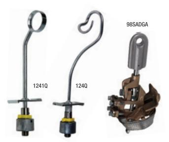
The **JUMPER HEADS** have a maximum opening of 19/16" (4.0 cm) and are designed with built-in universal joints in order to accommodate installation lines at an angle. The jumper heads have a quick action tightening screw for fast closing. Threaded adapters are used to accept 5/8-11 threaded non-shrouded ferrules. A hose clamp is included for connection strain relief.
