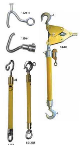
The **SECTIONALIZER KIT** temporarily disconnects and isolates a section of line without interrupting service to the balance of the circuit. The entire operation of installation and removal of the sectionalizers can be performed with live line tools. Particularly useful when circuits are interrupted as a result of conductor, insulation or pole failures. Service can be restored by cutting in sectionalizers to isolate the section of line that is in trouble.
