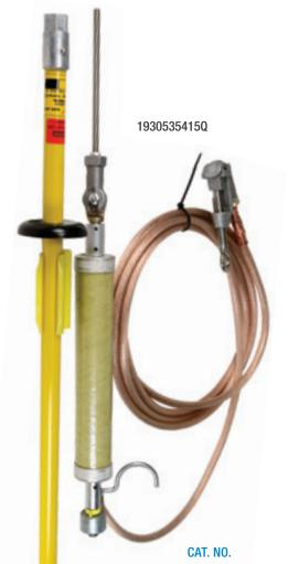
A **DISCHARGE HOOK** is used to drain capacitive voltage. The probe is first used to make contact, then the hook can be used to make direct contact bypassing the fuse. The fuse gives added protection in case initial contact is accidentally made on energized equipment. Fuse is rated at 8 kV maximum, 6 amperes continuous.
