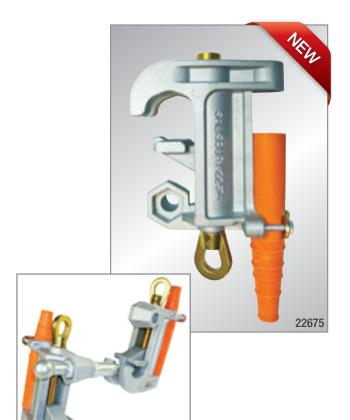
The **BALL AND SOCKET GROUNDING SYSTEM** allows for variable angle accessibility. This system is compact and lightweight. There are fixed grounding points on the socket clamp. The 21190 Socket Clamp, made from bronze alloy, has a socket size of 1 inch (25.4 mm) and a threaded bore boss of 5/8"-11 UNC. The socket clamp has an integral cable support with strain relief sleeve.
