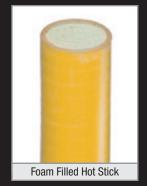
Hotstick production is 100% electrically proof tested. Hotstick blanks must pass a test of 100 kV/12" (305 mm) for 5 minutes without detectable heating prior to being accepted. Hot Stick blanks conform with ASTM F711 requirements.
