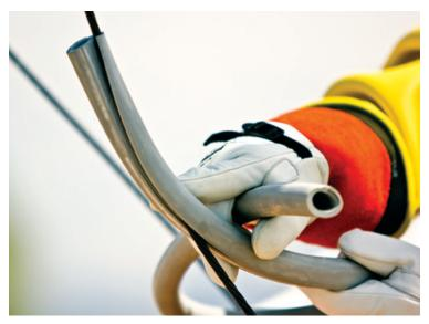
NOTE: INSTANT INSULATION IS CURRENTLY RATED AT 20kV PER ASTM D1050 18.2 ELECTRICAL FLASHOVER TEST. MATERIAL DIELECTRIC STRENGTH IS OF 486 V/MIL. EFFECTIVE THICKNESS IS .15" TO .2" WHEN INSTALLED.
