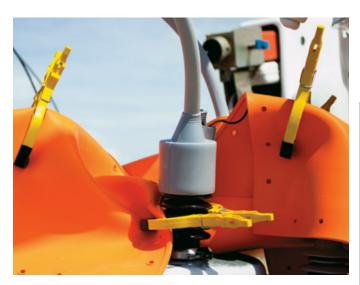
THE SALISBURY STINGER COVERS SC AND SCS SERIES ARE EXTRUDED IN EPDM OR SILICONE RUBBER AND DESIGNED FOR FIELD INSTALLATION OVER BARE CONDUCTORS. THE COVERS PROVIDE ELECTRICAL INSULATION AND PROTECTION FOR PHASE TO PHASE AND PHASE TO GROUND FLASHOVER THAT IS CAUSED BY WILDLIFE CONTACT. ACCEPTED BY (RURAL UTILITY SERVICES) RUS.
