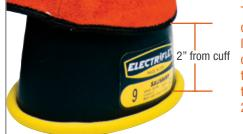
The minimum distance from the leather protector cuff to the bead of the rubber glove for this Class 2 glove is 2 inches.
