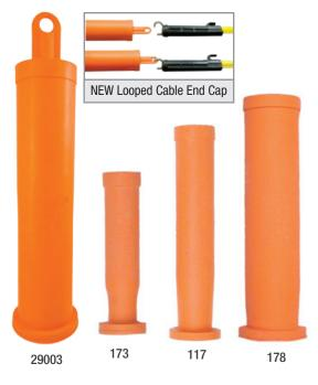
Cable End Caps are applied with rubber gloves. They are used on high voltage distribution cable ends found in vaults, cubicles and substations when cable remains energized during work. Cable End Caps are made from Type II orange SALCOR®.
