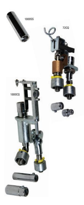
The **PARALLEL GROOVE CLAMP TOOL** accommodates cap-screw type parallel groove clamps (one, two and three bolt types). The parallel groove tool head clamps can be installed from almost any angle by use of the universal ball clamp. The handles are fiberglass, with the operating handle having a diameter of 1" (2.5 cm) and the stationary handle 1-1/4" (3.2 cm). Bag not included. Other lengths available.
