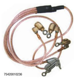
**SETS FOR GROUNDED "Y" SYSTEMS** provide all the equipment required to safely ground a variety of structures on grounded "Y" distribution systems. Factory assembled kits are for conductors ranging from #6 to 1-1/2" (3.8 cm) diameter, with serrated jaw "C" clamps with threaded terminals. All clamps are supplied with eye screws for installation with clampstick (not included). Other lengths and configurations are available.
