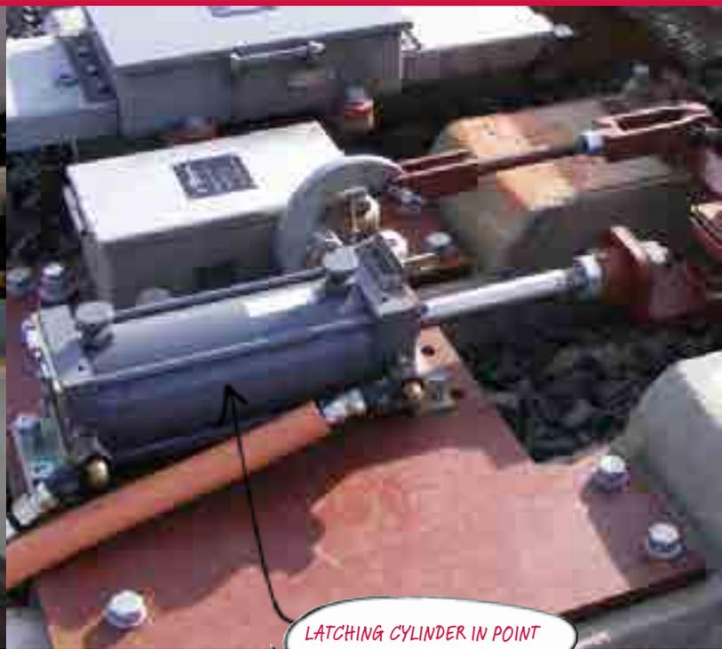
**LATCHING CYLINDER IN POINT SWITCHING SYSTEM**
