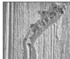
Figure 13. Contaminant embedded in the surface of a friction bearing
