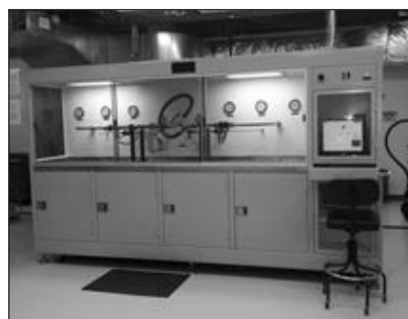
Fluid Care Center: Multi-Pass Test Stand
