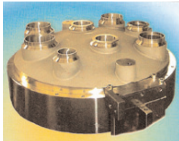
Figure 8. Dipole cryomagnet end cover HIPped from 316LN stainless steel powder operates in cryogenic environment of -268°C (-450°F). (photo courtesy of Bodycote HIP-Surahammer)
