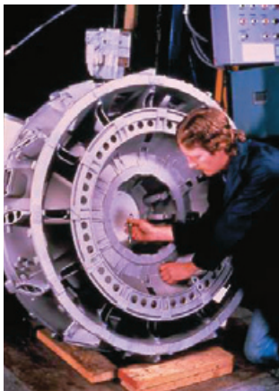
Figure 4. Castings are routinely HIPped to remove internal porosity.
