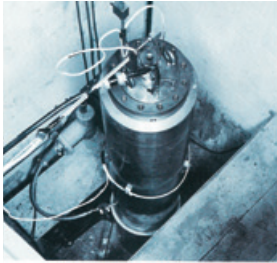
Figure 1. The first cold-wall gas pressure bonding vessel (now called HIP) installed and operated by Battelle in 1956.
