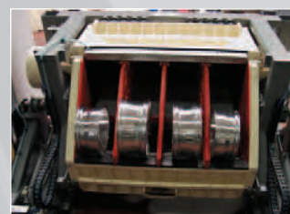
In the separating position: Processed components can be removed easily and new components can be added.
