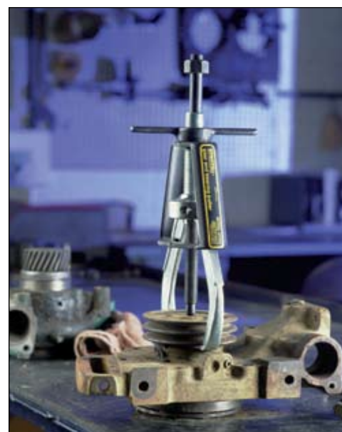
▲ EP-204 2-jaw puller positioned to pull a water pump drive pulley.
