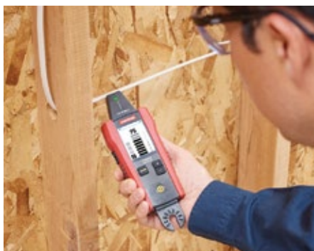
Trace energized and de-energized wires
