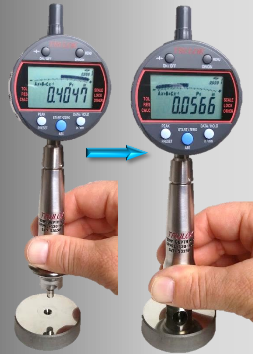
MHO-100-260 Countersink Angle: 100° Countersink Diameter: 0.2600" Thru Hole: .1250" Countersink Depth: 0.0566" Difference from Zero Preset: -0.0420"
