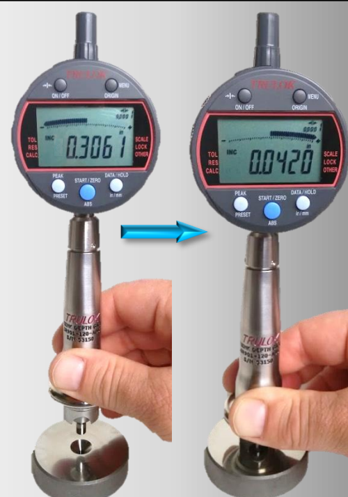
MHO-100-460 Countersink Angle: 100° Countersink Diameter: 0.4600" Thru Hole: .1250" Countersink Depth: 0.1406" Difference from Zero Preset: +0.0420"
