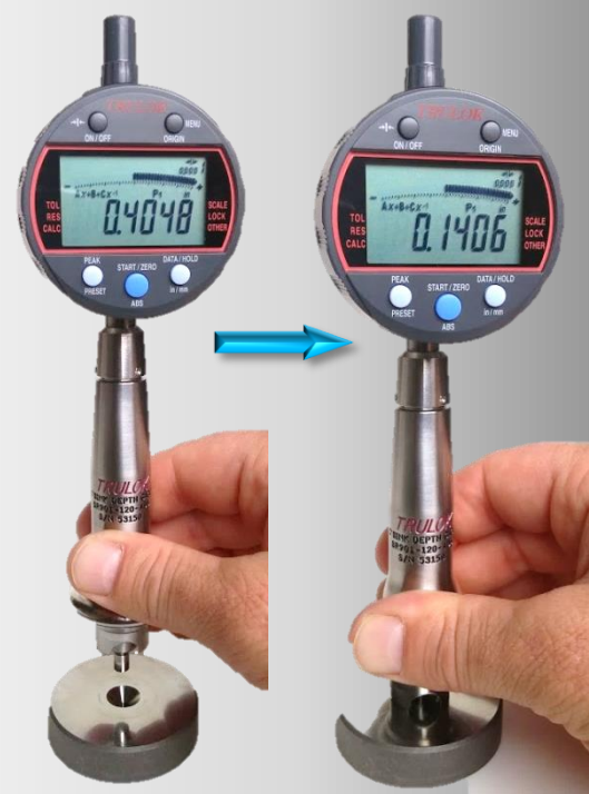
MHO-100-460 Countersink Angle: 100° Countersink Diameter: 0.4600" Thru Hole: .1250" Countersink Depth: 0.1406" Difference from Zero Preset: +0.0420"
