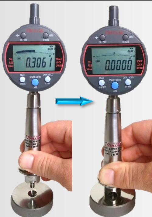
MHO-100-360 Countersink Angle: 100° Countersink Diameter: 0.3600" Thru Hole: .1250" Countersink Depth: 0.0986" Difference from Zero Preset: 0.0000"
