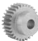
22400-20 Spur gears stainless steel, module 1.5 toothing milled, straight teeth, engagement angle 20°
