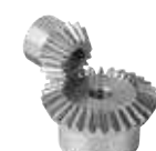
22430 Bevel gears in steel, ratio 1:2 toothing milled, straight teeth, engagement angle 20°
