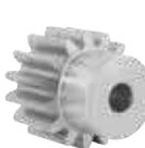
22400-20 Spur gears stainless steel, module 3 toothing milled, straight teeth, engagement angle 20°
