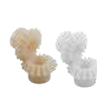
22432 Bevel gears, plastic, ratio 1:1 injection-moulded, straight teeth, engagement angle 20°
