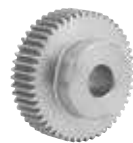
22400-20 Spur gears stainless steel, module 1 toothing milled, straight teeth, engagement angle 20°
