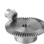
22430 Bevel gears in steel, ratio 1:4 toothing milled, straight teeth, engagement angle 20°
