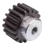
22401 Spur gears steel, module 4 toothing hardened, straight teeth, engagement angle 20°
