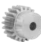
22400-20 Spur gears stainless steel, module 2.5 toothing milled, straight teeth, engagement angle 20°
