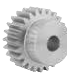
22400-20 Spur gears stainless steel, module 2 toothing milled, straight teeth, engagement angle 20°
