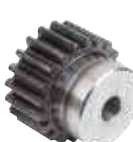
22401 Spur gears steel, module 2.5 toothing hardened, straight teeth, engagement angle 20°
