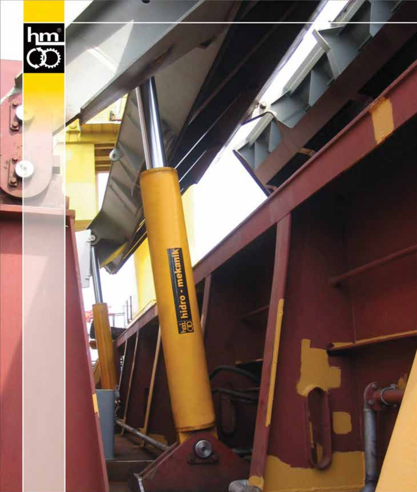
HATCH COVER HYDRAULIC SYSTEM
