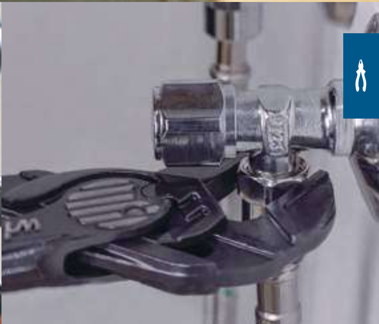
Quick fastening thanks to the ratchet function
