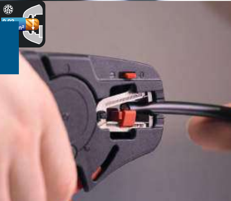
Large insulated area from 0.03 - 16 mm 2 .
