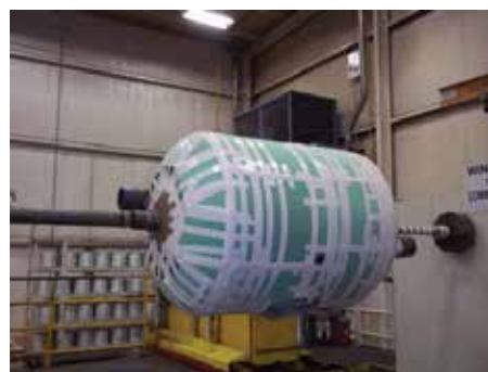
Insulated Vessel at Start of Winding
