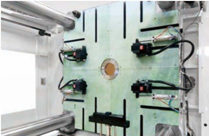
6,500kN (650ton) IMM vertical loading Die setting system & Hydraulic clamp, automatic slidable type TYC100Z
